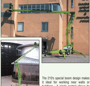
The 210's special boom design makes it ideal for working near walls or buildings. A single control allows its platform to move vertically while remaining parallel to the job, saving time and improving efficiency.
